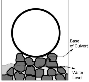
Installing a culvert above the existing streambed creates a serious barrier to fish and wildlife movement. When the culvert is higher than the surrounding streambed it is often refered to as "perched".
